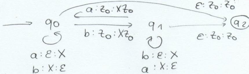
$Q = \{q_0, q_1, q_2\}$   $\Sigma = \{a, b\}$   $\Gamma = \{z_0, X\}$   $F = \{q_2\}$
