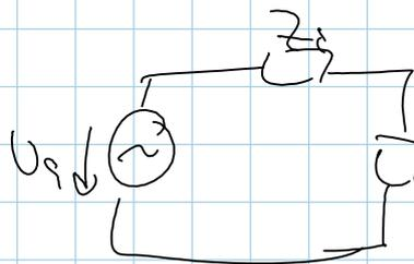
$$z_E = z_i^* \quad \text{mit } z_i = (1+j)50 \Omega \quad l=l_1$$
