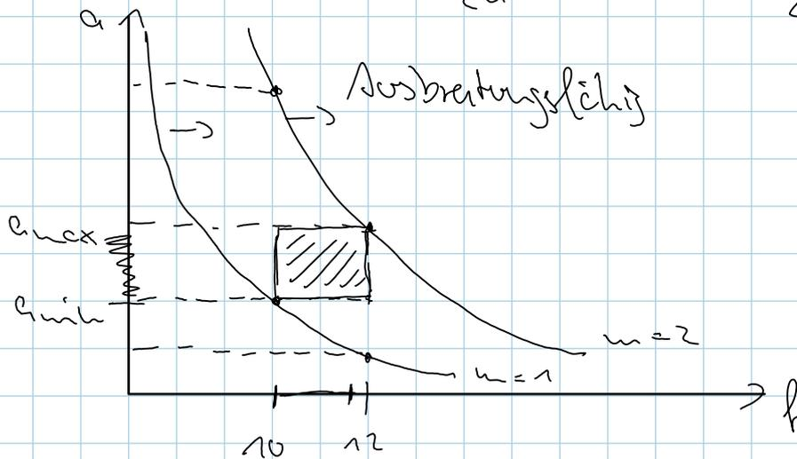
m=1:  $a(f_{c10} = 10 \text{ GHz}) = 1,5 \text{ cm} = a_{\min}$
