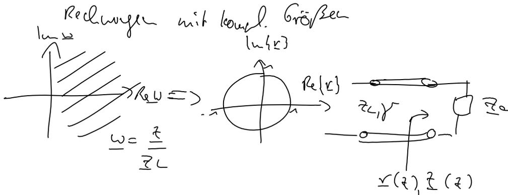
$$c.) \quad \underline{z}(z) = \frac{z(z) - z_L}{z(z) + z_L} = \frac{\underline{w}(z) - 1}{\underline{w}(z) + 1}$$
