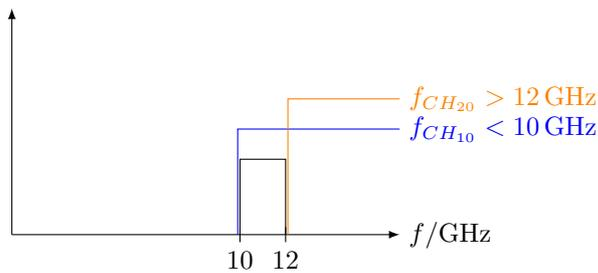
$$\begin{aligned} \frac{c_0}{2a} &= f_{CH10} \leq 10 \text{ GHz} \\ \Rightarrow a &\geq \frac{c_0}{2f_{CH10}} = 15 \text{ mm} \\ \frac{c_0}{a} &= f_{CH20} \geq 12 \text{ GHz} \\ \Rightarrow a &\leq \frac{c_0}{12 \text{ GHz}} = 25 \text{ mm} \end{aligned}$$
