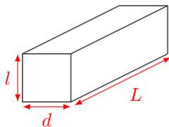
$$\begin{aligned} \underline{Z}_{\square} &= \frac{\underline{E}_z(x = \pm \frac{d}{2}) \cdot l}{\underline{I}} \\ &= \frac{\beta}{2\sigma} \cdot \frac{1}{\tanh\left(\frac{\beta d}{2}\right)} \end{aligned}$$
